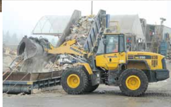
(Above) This United Recycling operator uses a Komatsu PC300LC-7 to feed wood waste into a grinder. (Left) United has three Komatsu WA250 wheel loaders to handle construction and demolition debris.
